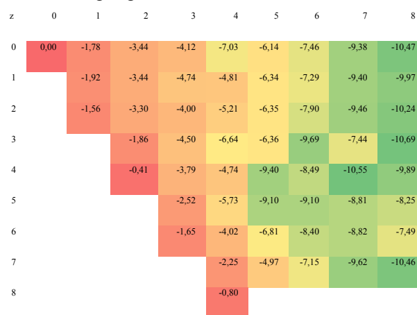
Figure 2. Free energy (eV, at 500K and water saturation pressure) of the most stable configuration obtained according to the number of water molecules adsorbed on the nanoparticle (horizontal axis) and the number of broken bonds on the water molecules (vertical axis), i.e. the degree of water dissociation.
